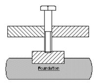
They have one in each corner of the machine and by turning the bolt it will either raise or lower that corner. The Japanese wanted to leave instructions for the Aussie night shift fitters and so they taped a piece of paper with the message "please take jacking screws out".
